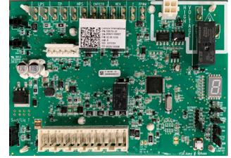
**NOTE** - Two RAST connectors for a conventional heating/cooling thermostat are also provided for connecting to the control. A two-stage or single-stage thermostat can be used.
